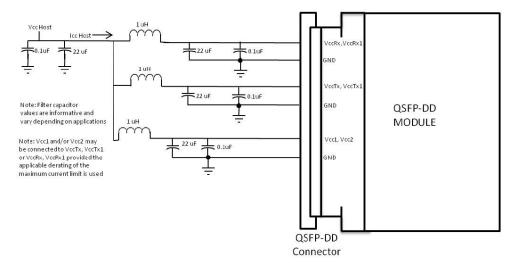
Figure 3. Host Board Power Supply Filtering
