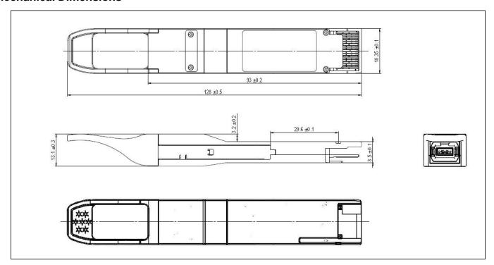
Figure 10. Mechanical Specifications
